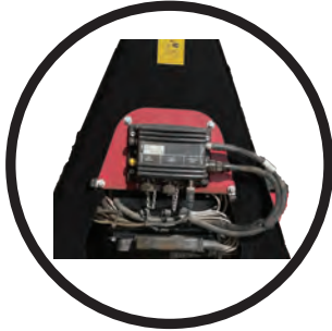
Hydraulic control valve inserted inside the frame
